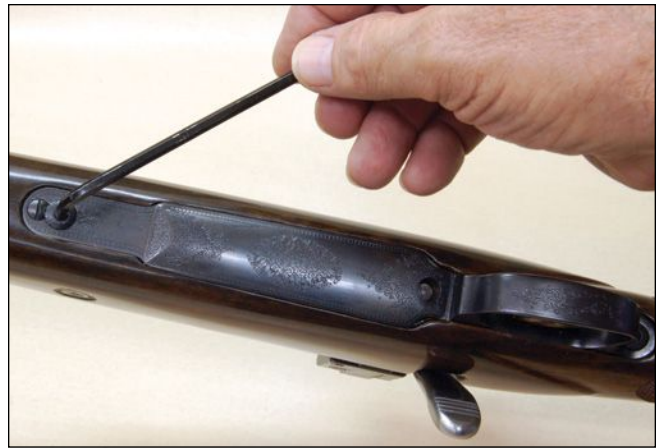
Socket-head guard screws can be tightened or removed (no matter how tight) with just one hand on the rifle and one on the wrench.
