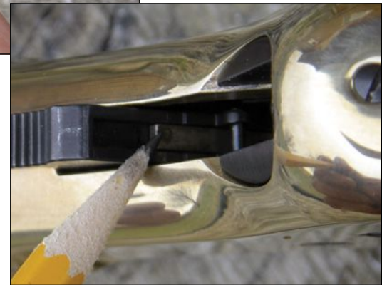
The Big Boy hammer features a transfer bar that must be managed correctly.
