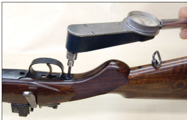
Socket-head guard screws are usually mandatory to prevent the driver bit from slipping off the screw when using a torque wrench to firmly tighten them.
