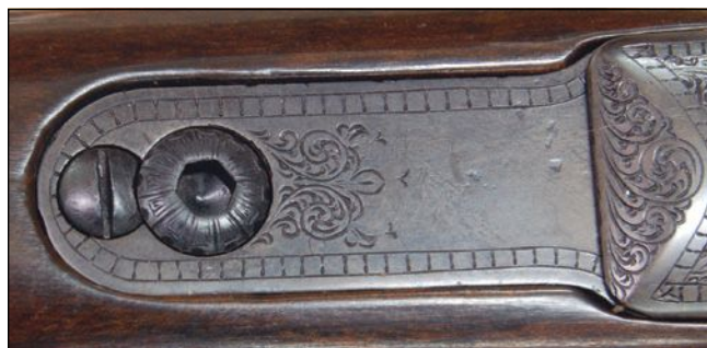
Socket-head screws don't have to be plain; engraving adds to their appearance.
