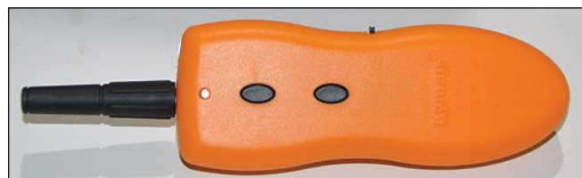
The handheld remote control uses a 9-volt battery.
