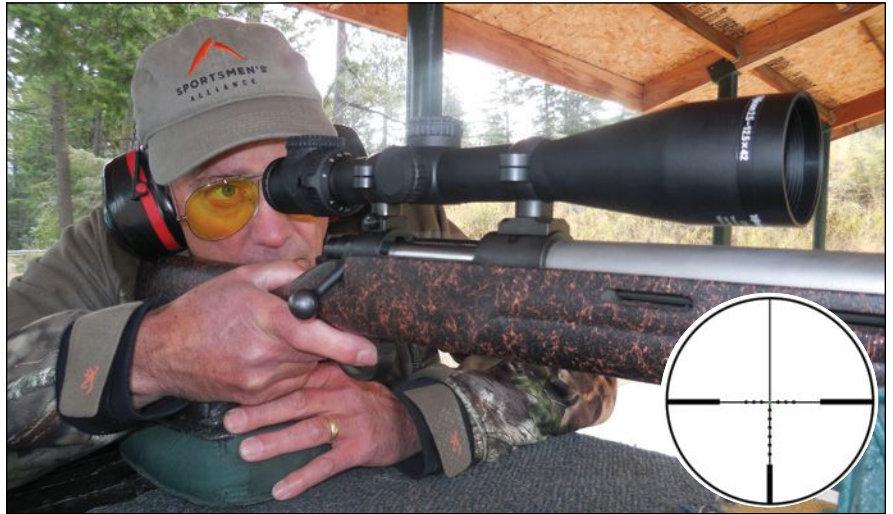
A Cooper Model 22 .243 Winchester was used to test a Trijicon AccuPoint 2.5-12x 42mm riflescope with an MOA-dot crosshair reticle.
