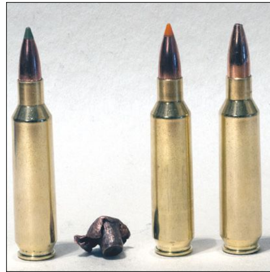
Bullets tried in the Heritage rifle include (left to right): the Nosler 55-grain E-Tip shown with a bullet recovered (47.1 grains) from a pronghorn, a 55-grain Ballistic Tip Varmint boat-tail and a handloaded Barnes 50-grain Varmint Grenade hollowpoint.
