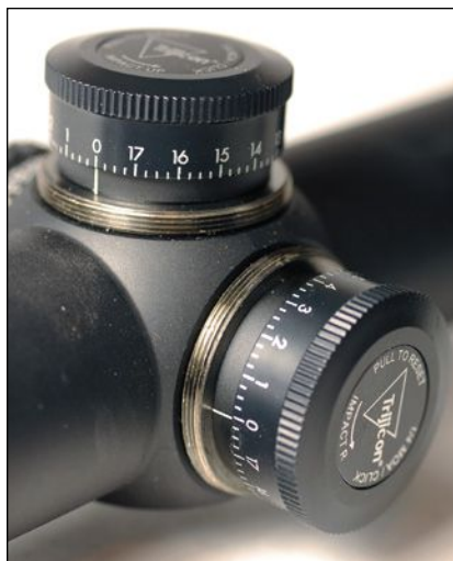
Windage and elevation turrets allow adjustments of 90 minutes of angle. The dials can be pulled out and reset to zero.
