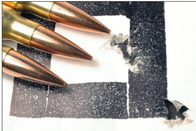
Right, a 100-yard group shot with Federal Premium Gold Medal Berger 185-grain Juggernaut OTM loads.
