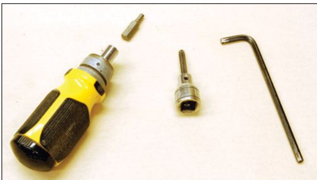
Drivers for socket-head guard screws include (left to right): insert bits for magnetic screwdrivers, heavy duty ratchet wrenches for 3/8-inch drives and a common L-shaped Allen wrench.
