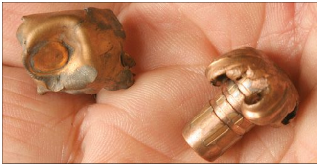
These .30-caliber bullets were recovered from mule deer bucks. The “traditional” bullet (left) did not make it through the ribs on a broadside shot. The Barnes TSX (right) entered the flank of a big buck angling almost directly away and was found under the hide on the front of the chest.
