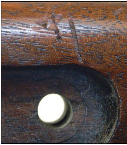
Scratches on this old Springfield stock show signs of a screwdriver slipping out of the screw slot.
