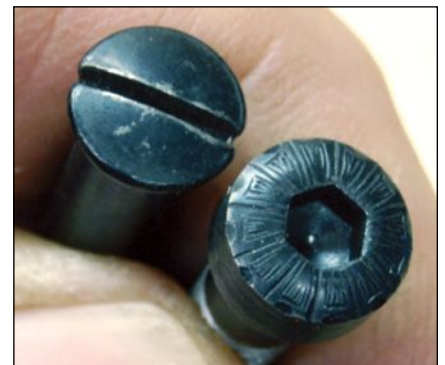
A slotted guard screw (left) as compared to a socket-head screw.
