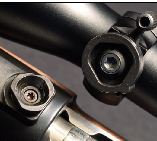
The detachable mounts are sleek, unobtrusive and quick to operate. The receiver will accept standard bases for a large-ring Mauser action.
