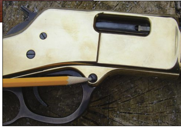
The lever pivots from a single screw, resulting in fast and smooth operation, but also allows easy removal of the lever and bolt for barrel breech cleaning.
