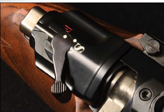
The bolt shroud is nicely sculpted and features a Model 70-style, three-position wing safety. It is crisp, smooth and snaps into place at each stage.
