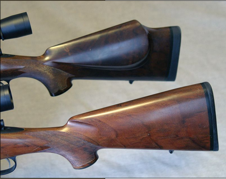
The stocks above were made by the same custom stockmaker for two different customers, and fit each shooter so well felt recoil was noticeably reduced – unless they shot each other’s rifle. Right, the stocks of most big-game rifles once had relatively hard rear ends, like the steel buttplate on this custom stock that increases felt recoil considerably.
